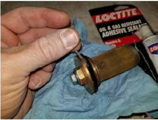
**The failed gasket sealant.**
