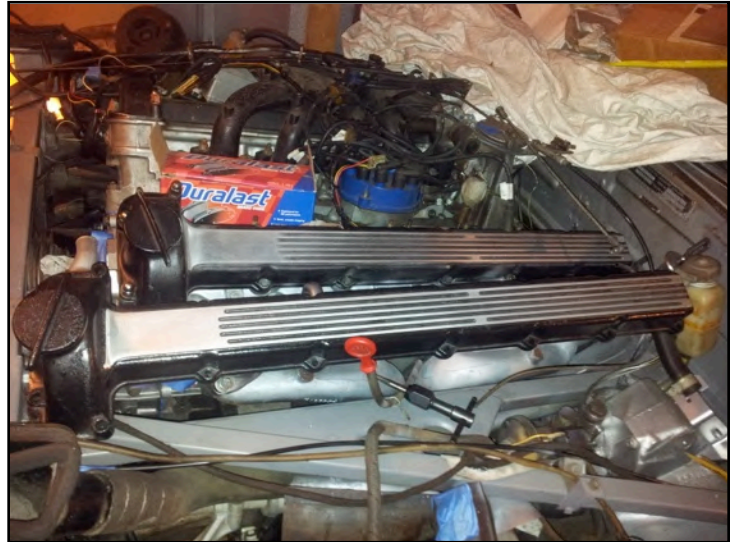
Cam Cover Refinishing In Progress
