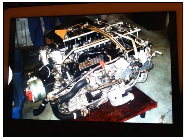
Jaguar V12 with air rails visible
