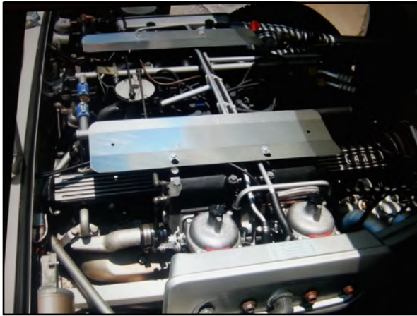
Rain shields hiding air rails
