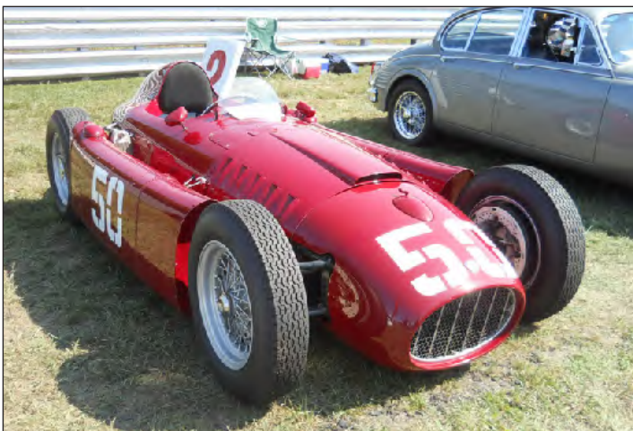
Driver safety was not a big issue in the 1950s, as this Lancia D50, F-1 car illustrates with its pannier fuel tanks.
