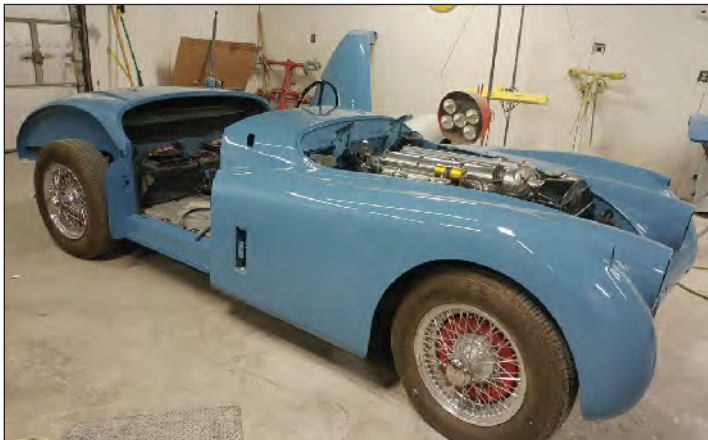
Reassembly begins after painting.
