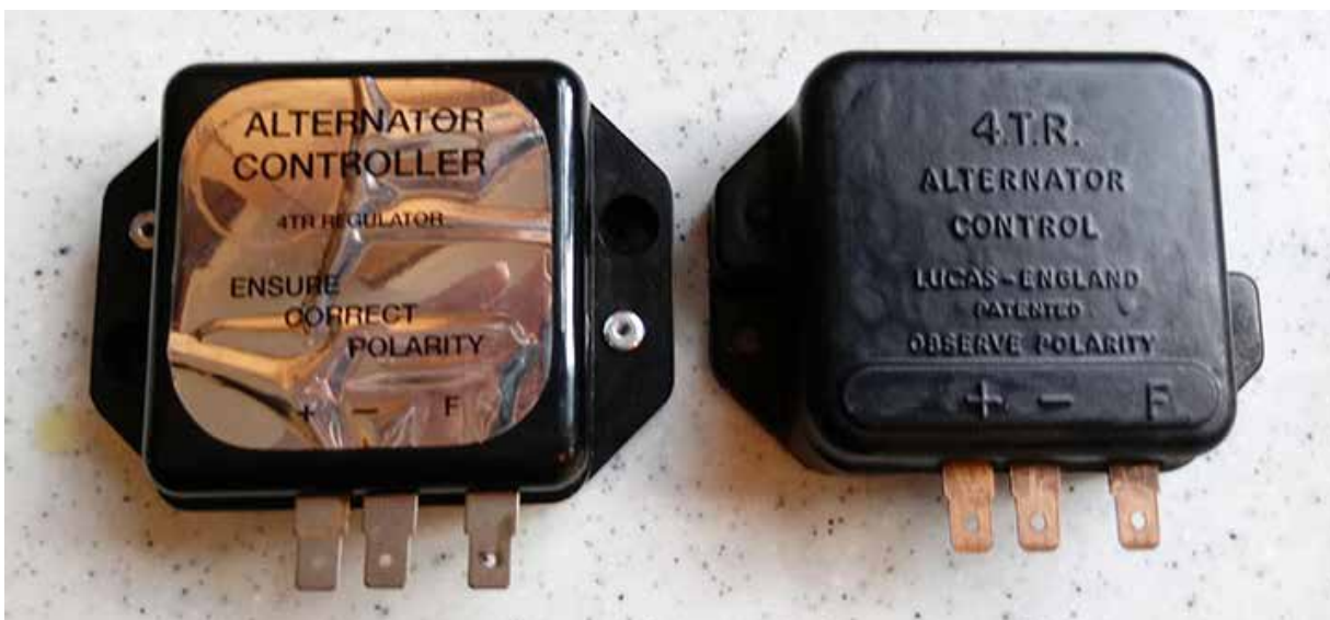
Sometimes bodge jobs look better than original equipment. Former VJC President Davis Harrison submitted this photo of an original part, at right, and the more modern looking aftermarket replacement at left.
