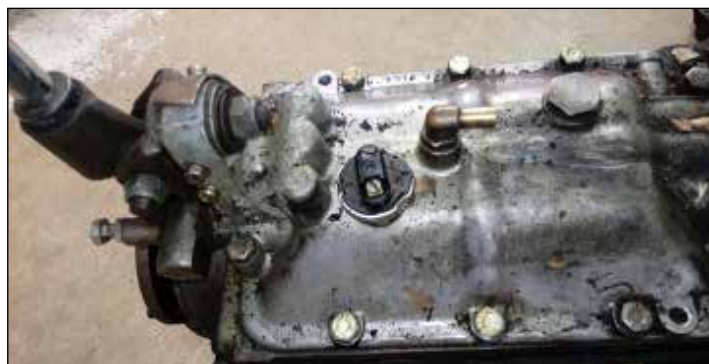
The old gearbox top shows bodedged repair.
