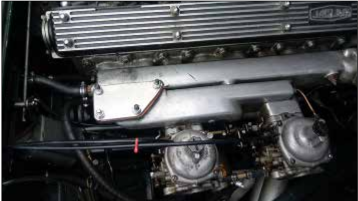
Temporary manifold hump.
