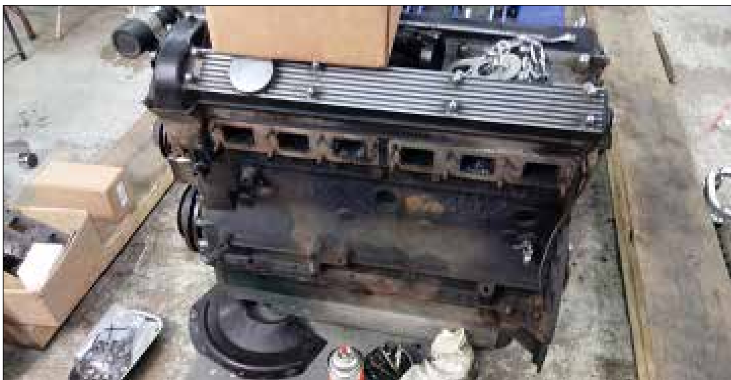
The E-Type's engine before cleaning and painting.
