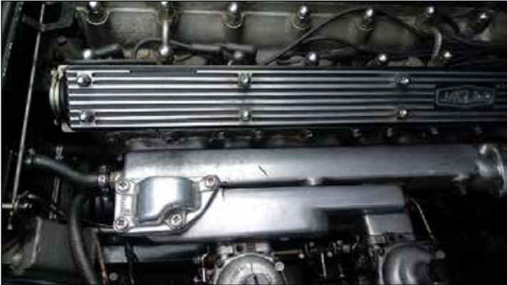
Proper factory manifold hump.
