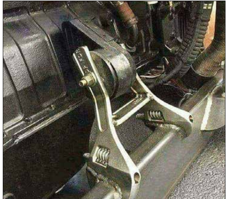
When you need a motor mount and all you have is a toolbox and a welding torch, improvise. (Contributed by David Harrison, VJC)
