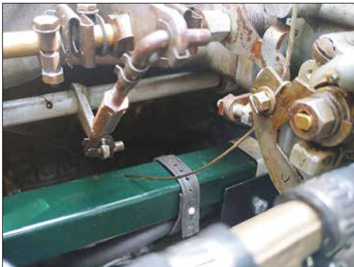
Adjustable link to Strombergs.
