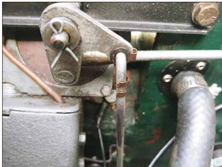
Carb side bell crank, correct degree of leverage.
