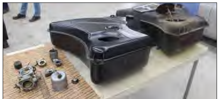
A dismantled E-Type gas tank at right, alongside a replacement aftermarket tank.
