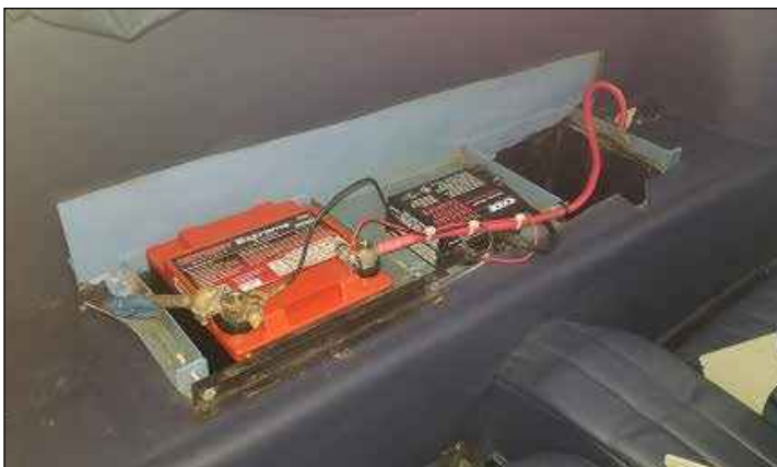
Modified Odyssey PC925 sealed battery installation.
