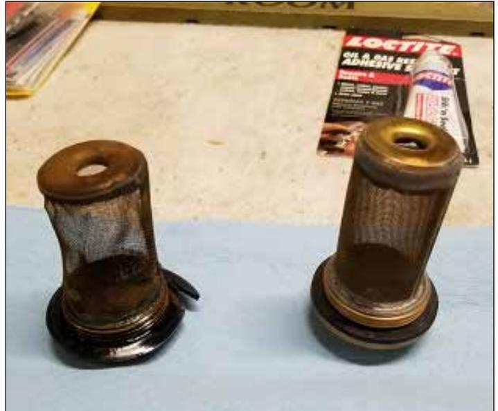
**The old (left) and new drain plugs with attached mesh filters.**
