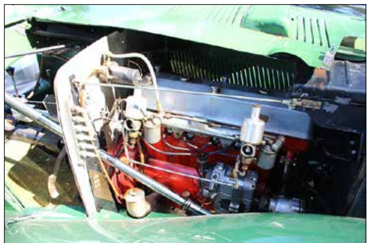
An MG 6-cylinder engine complete with magneto ignition.
