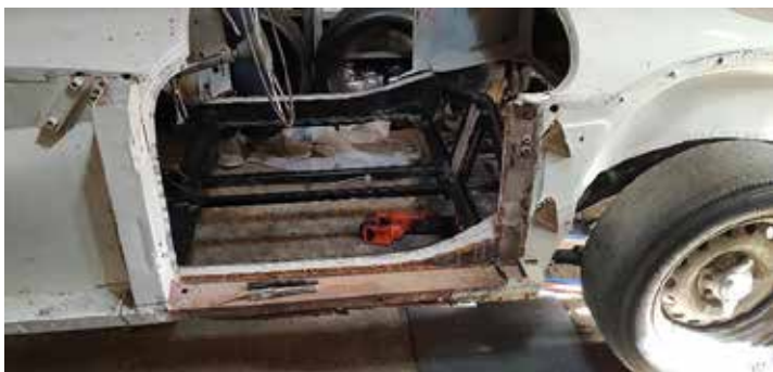
The dreaded "tin worm" had been nibbling away at the MG's doorsills.
