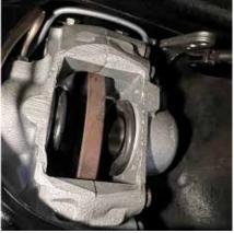
pers. The parking brake mechanism is bolted to the caliper and cannot be removed while still in the rear cage, unless disassembled from the calipers, and extracted seperately. Further complicating the job, wait until you see how difficult it is to get out the two bolts securing each of the calipers.
